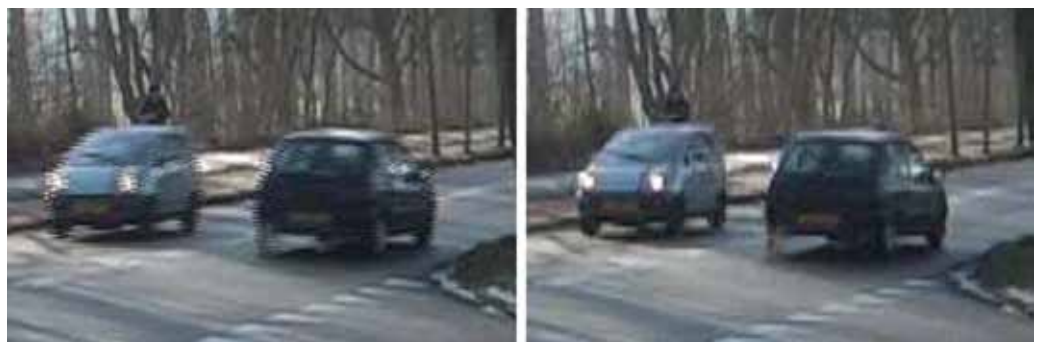
Figure B5.5. The left image is the blurred image of the original recording; the right image the de-interlaced image (50 images per second)
